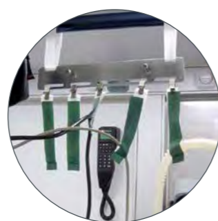
Clip-Fix 3 Guiding and holding of the breathing circuit and the cable systems at the service rail placed on the handgrip of the rescue vehicle.
